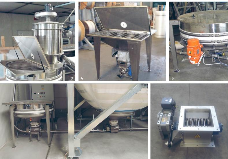
1 Dump stations with minisilos 2 Diaphragm valve 3 Antidust filter 4 Dump station with lump breaker for sugar 5 Vibrating cone 6 Dump station with silsystem 7 Lump breaker
