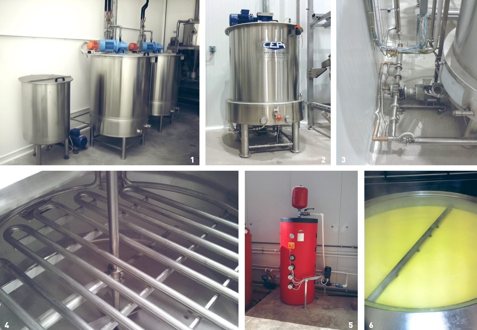
1, 2 Dissolving tank with heated bottom 3 Pompa 4 Heated coil 5 Boiler 6 Heated product
