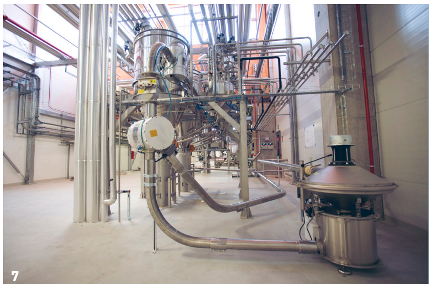
1 Extraction with vibrating cone 2 Magnet in pneumatic line 3 Extraction in direct suction 4 Trevira fabric 5 CEPATIC safety system 6 Silo weighing 7 Vibrosifter
