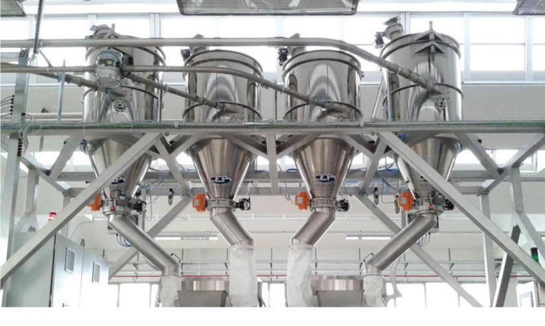
Self-cleaning filter (1) Dust exhaust unit with lid (2) Weighing cells (3) Discharging valve (4) Antidust (5) Level sensor
