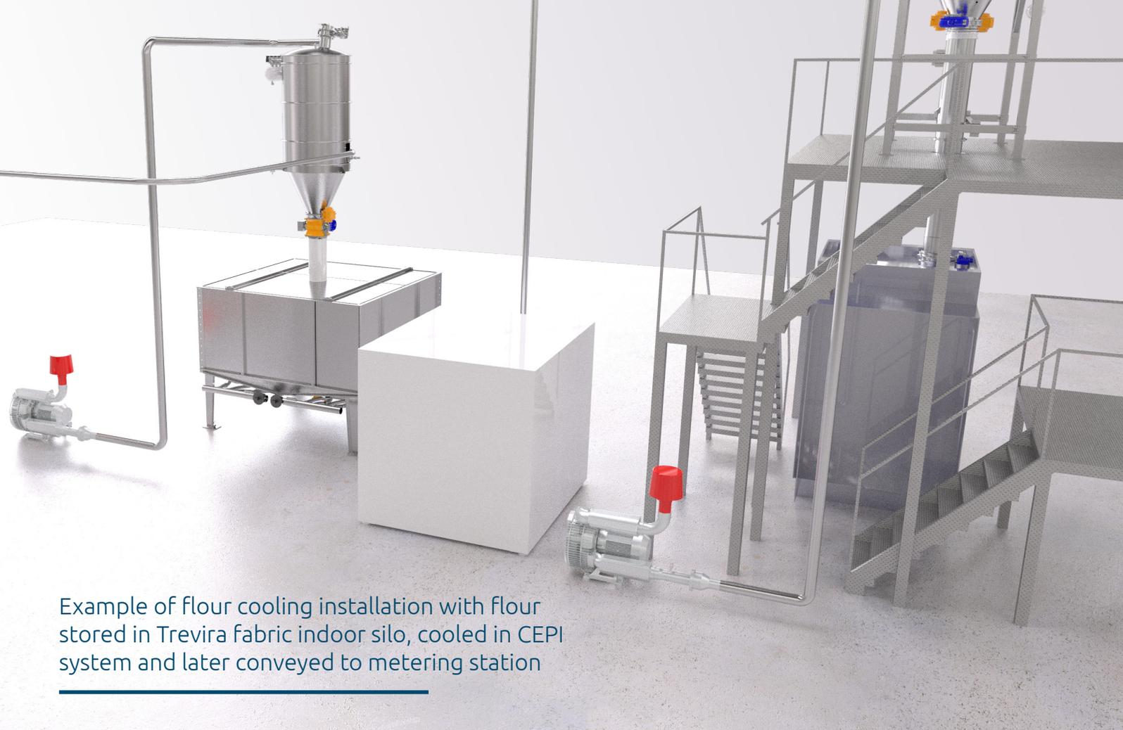
Example of flour cooling installation with flour stored in Trevira fabric indoor silo, cooled in CEPI system and later conveyed to metering station
