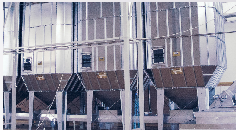
Installation with silbox silos, microingredients stations and invert sugar system; Silos for cous-cous
