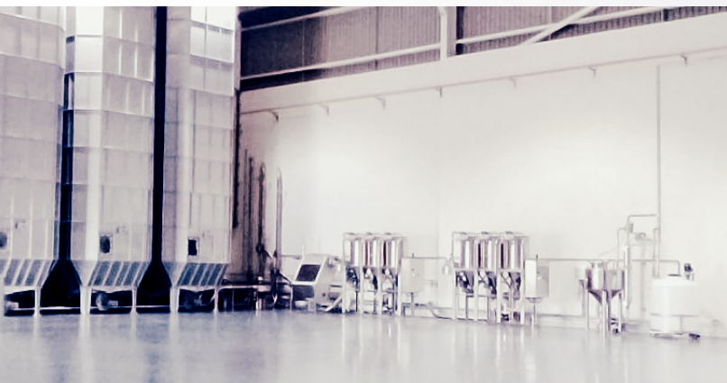
Installation with silbox silos, microingredients stations and invert sugar system; Silos for cous-cous
