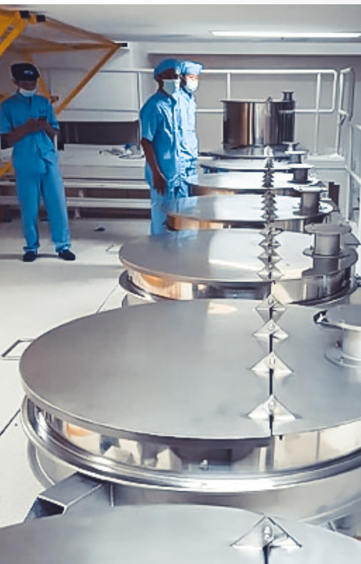
Left to right, top to bottom: storage hoppers with raw materials dumping, continuous vibratory feeder (up to eight feeders)
