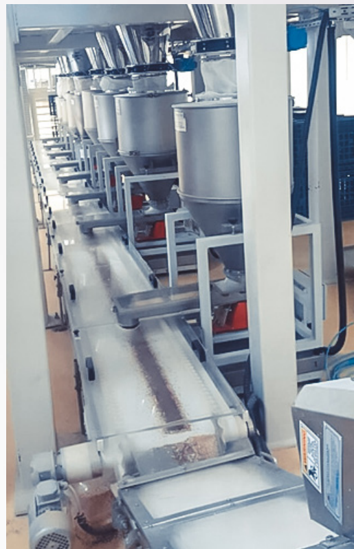
Left to right, top to bottom: storage hoppers with raw materials dumping, continuous vibratory feeder (up to eight feeders)
