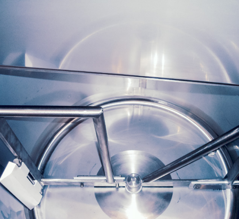
Scraper with adjusted speed, to gently work the raw materials into the tank and avoid clumps
