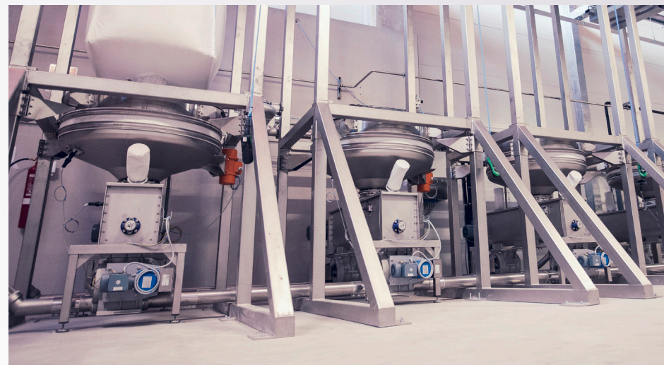
Left to right, top to bottom: chain hoist to lift the bags; antidust filter; sifting system; multiline feeding
