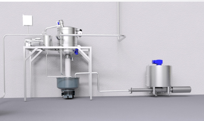
Dosing station and cold dosing tank
