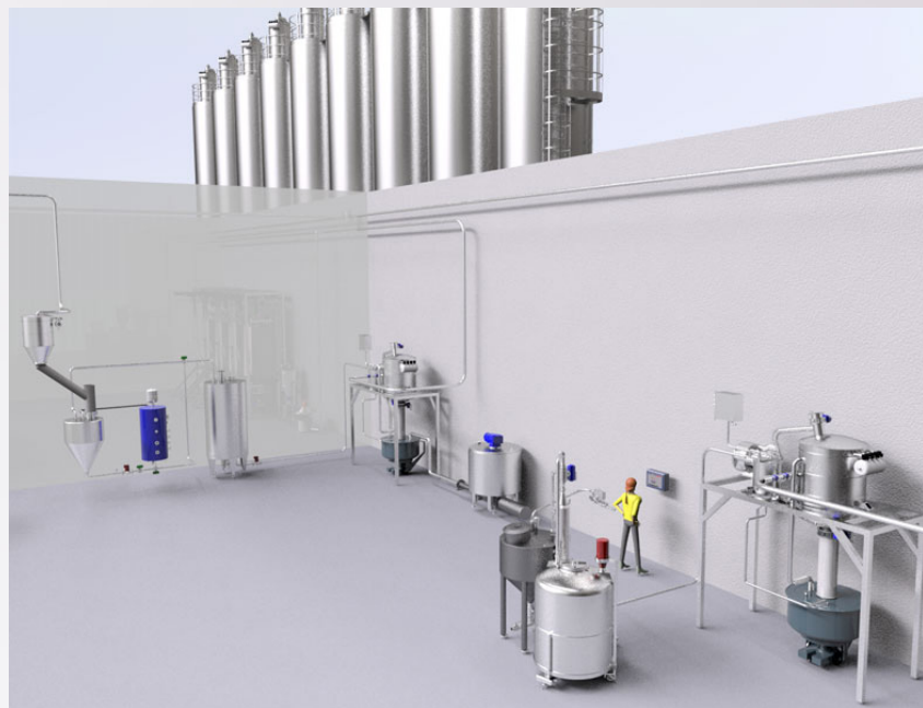
Dosing area: one station with sugar invert system and cold fat metering and one station with salt solution
