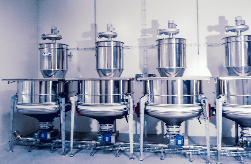
Storing of medium ingredients in dump station battery; Anti-dust filter
