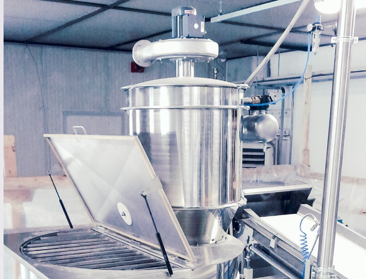
Storing of medium ingredients in dump station battery; Anti-dust filter
