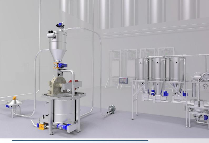
Sugar mill with in-line sifter in controlled environment room with microingredients station and touch panel
