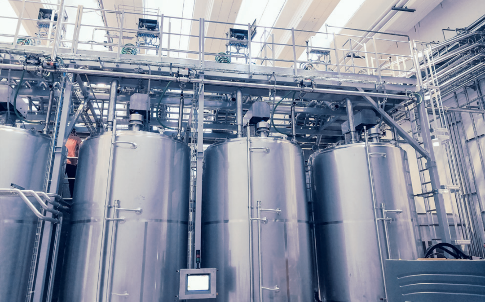
Fully automated sourdough preparation group for big production volumes, with PLC control
