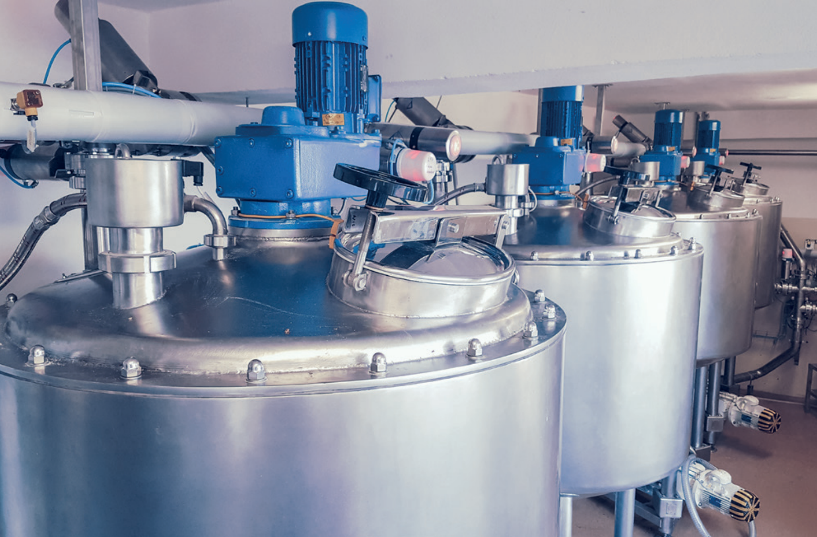
Sourdough preparation group for medium production volumes. Above: detail of stirrer and inspection hatch. Below: dosing system with total emptying
