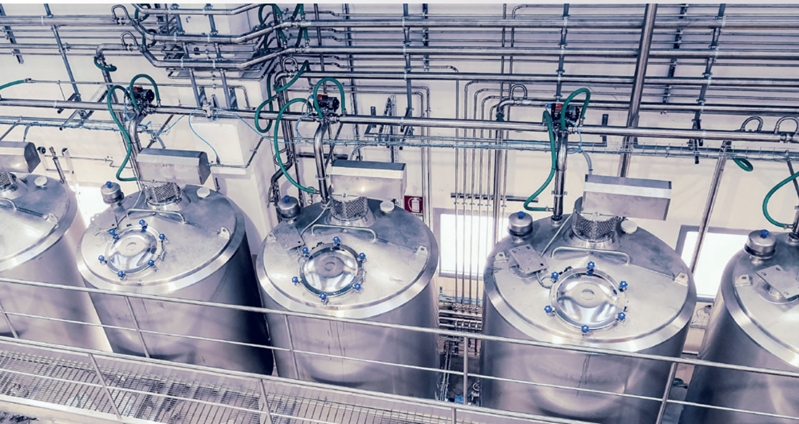
Fully automated sourdough preparation group for big production volumes, with PLC control
