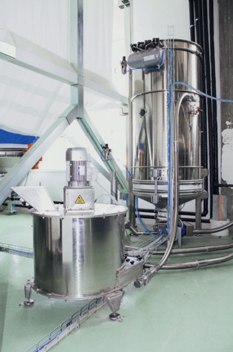
Biscuit rework system and cutting mill detail
