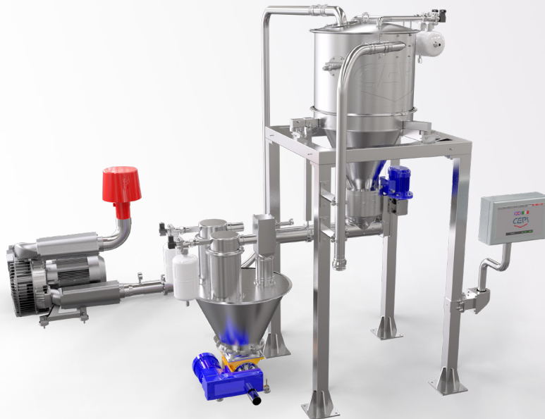
Continuous metering station
