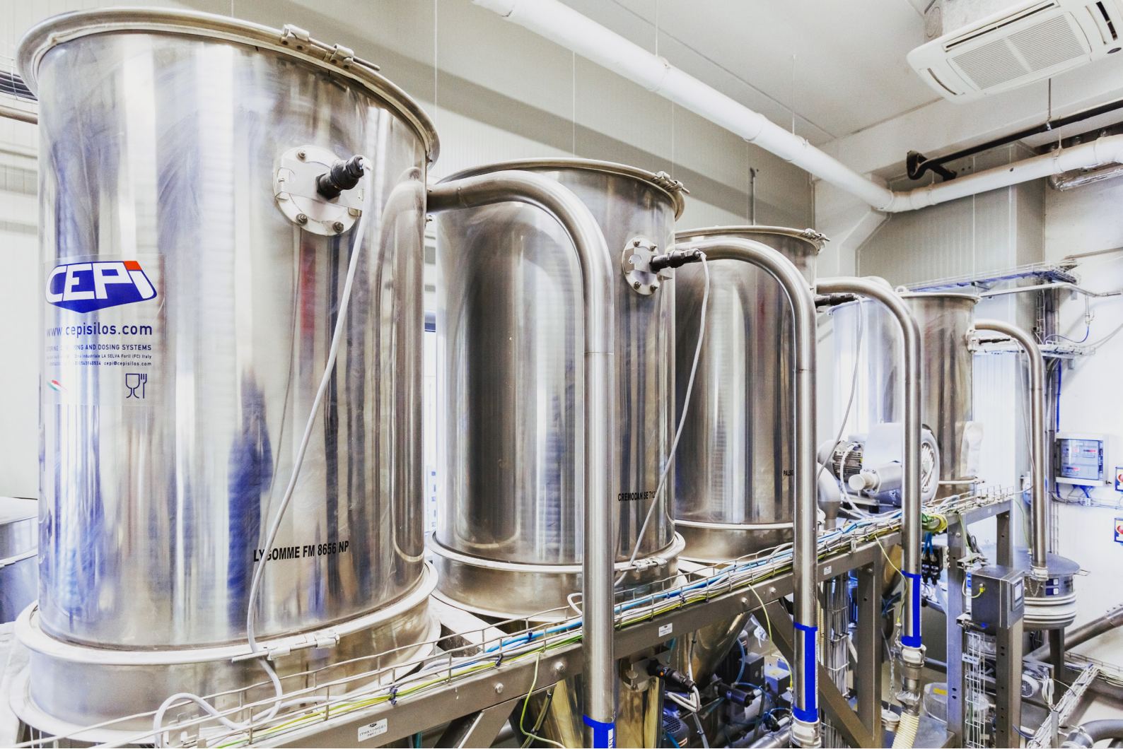
Microingredient station; Details: capacity probe, loading system
