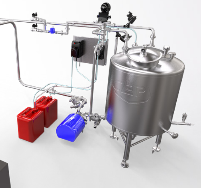
Detail: storing and dosing of water, detergent and sanitizer
