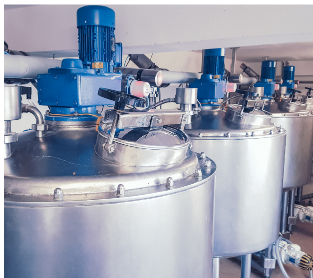
Fully automated sourdough preparation group for medium production volumes. With PLC control.
