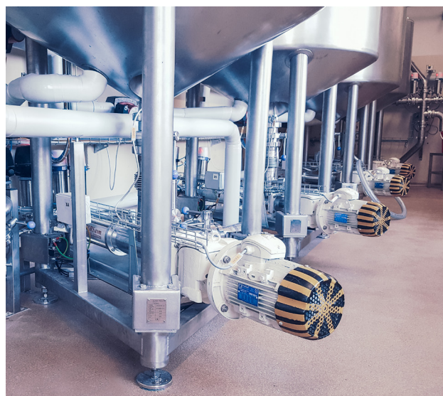
Sourdough preparation group for medium production volumes. Left: stirrer and inspection hatch. Right: dosing system with total emptying
