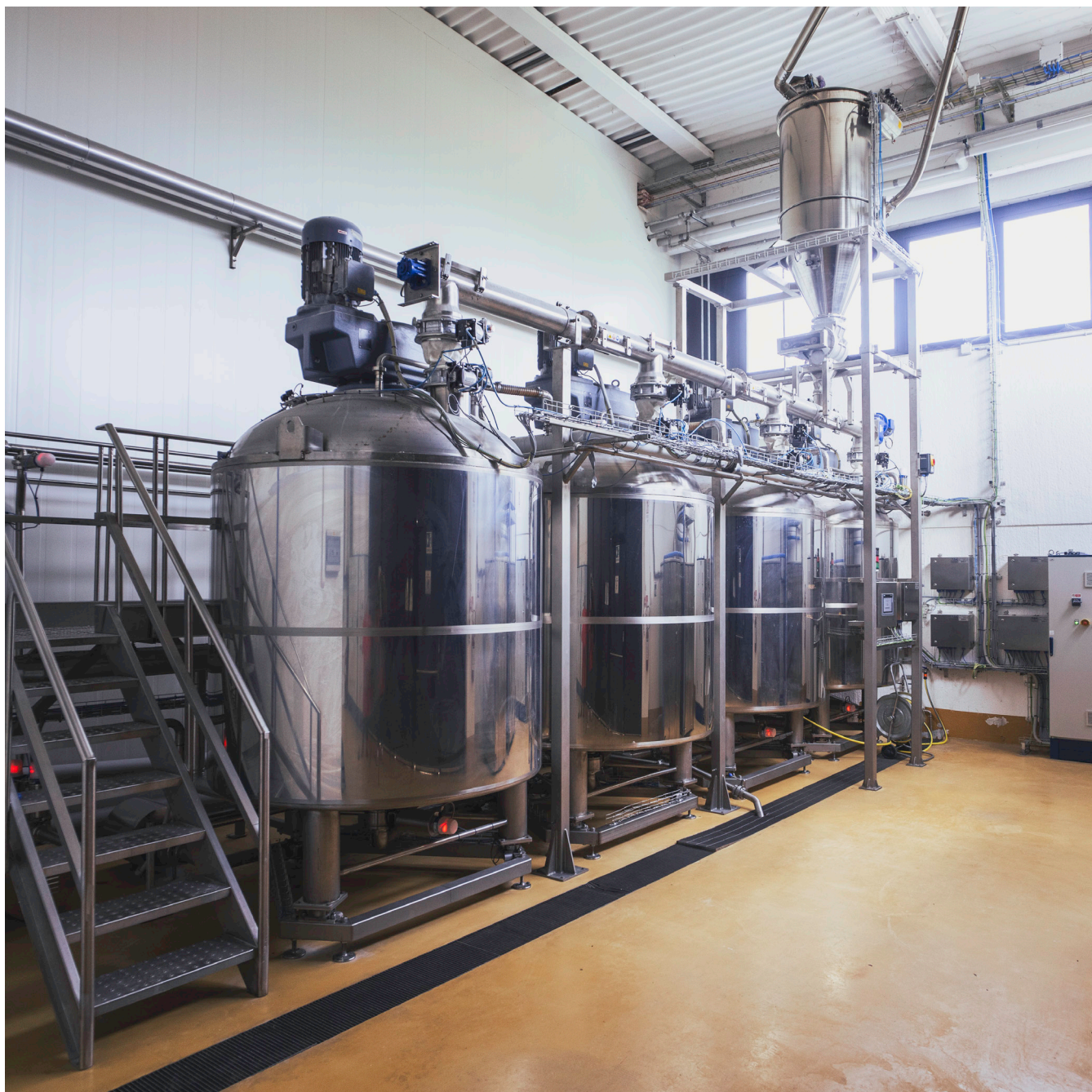
System for the preparation, storing and dosing of sourdough.
