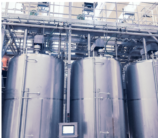
Fully automated sourdough preparation group for medium production volumes. With PLC control.
