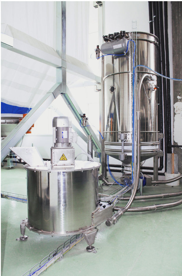
Biscuit rework system and cutting mill detail
