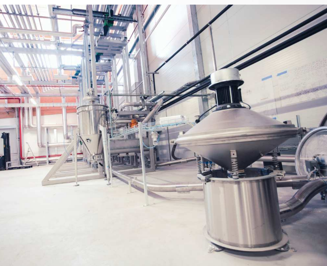
Left to right, top to bottom: chain host to lift the bags; antidust filter; sifting system; multiline feeding
