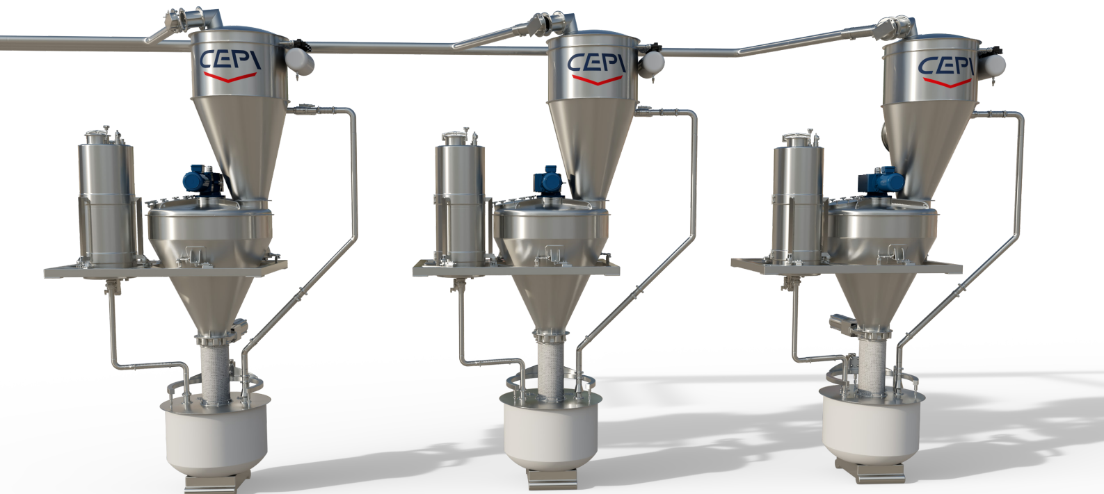
Three blenders dosing on separate mixers
