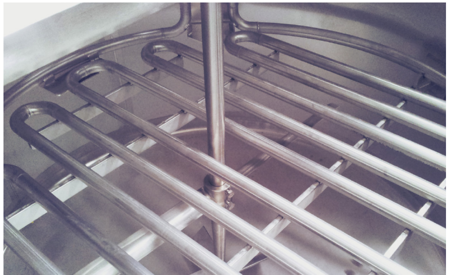
Heated coil. Left: boiler.
