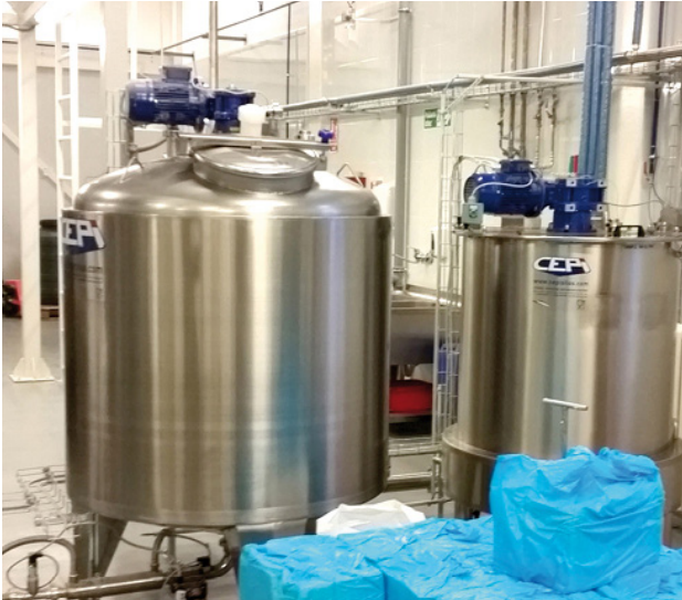
Fat tank with agitator and inspection hatch. Right: heated bottom detail.
