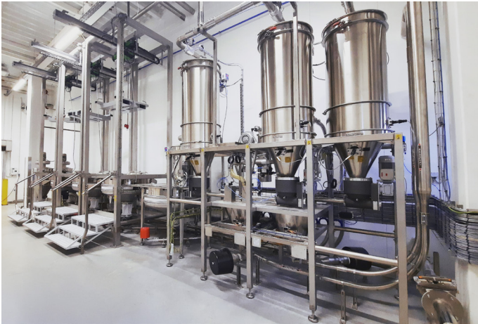
Microingredients stations fed by Big Bag systems and Dump stations
