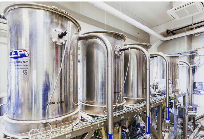
Details of microingredient station: capacity probe, loading system (left) and dedicated HMI (right)
