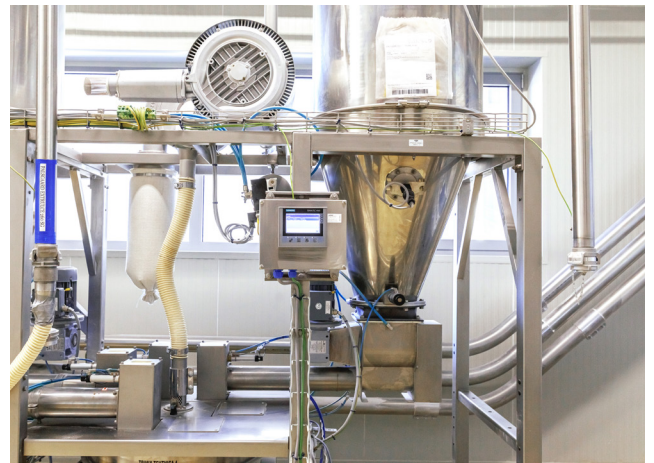
Details of microingredient station: capacity probe, loading system (left) and dedicated HMI (right)
